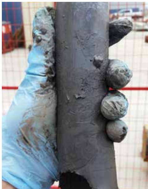
Sample cores of the treated material are being analyzed for geotechnical properties to determine suitability for reclamation activities.
